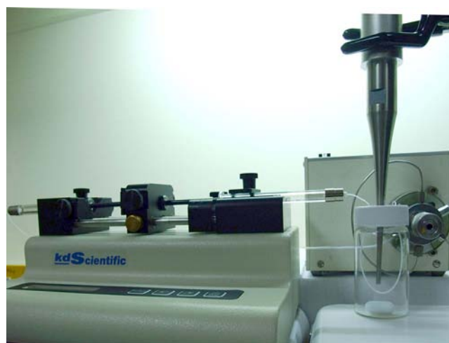
Figure 1. Photograph of the proposed UA-PPP-HF-LPME system.
